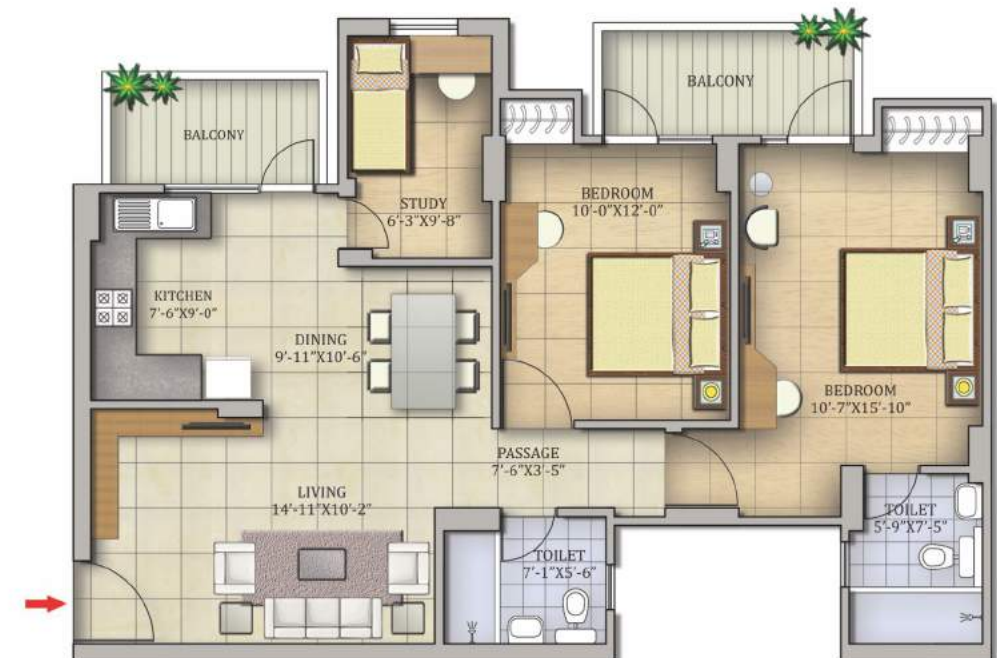
UNIT - 1 2 BEDROOM + STUDY + 2 TOILET CARPET AREA = 74.784 SQM. (804.974 SQ.FT.) BALCONY AREA - 9.520 SQM. (102.473 SQ.FT.) BUILT UP AREA = 90.820 SQM. (977.586 SQ.FT.) SUPER AREA = 122.632 SQM. (1320.00 SQ.FT.)
